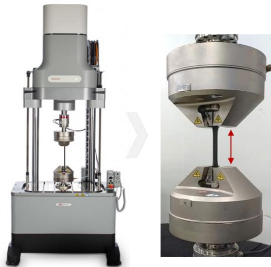
Electrodynamic fatigue testing system Model : ElectroPuls E10000 (Instron) Load / Stroke : 10 kN / 60 mm
