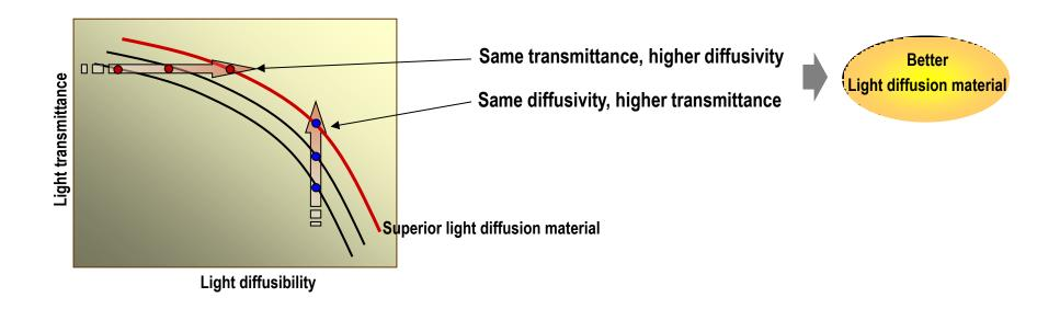
→ Comparison of light diffusing materials : Need to review both transmittance and diffusivity
