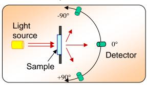
• HA: angle at which half amount of light flux is measured
